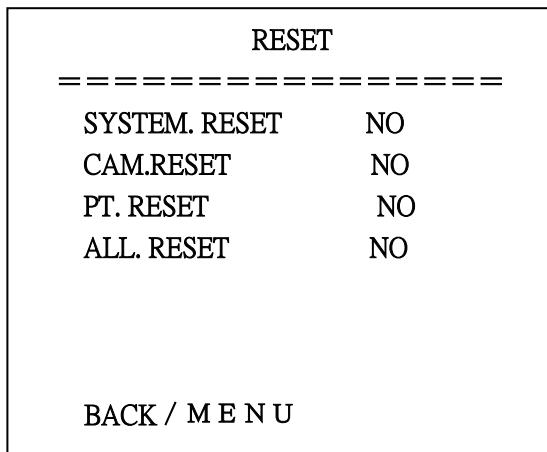
**SYS. RESET:** system reset:Protocol: VISCA; Address: 1; baud rate:9600; RS485:Off
