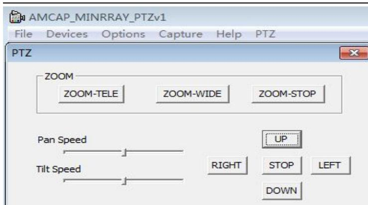
9. When the camera is power-on and begin initialize, horizontally to the left turn to the limit position, vertically turn to the bottom; finally both horizontal and vertical turn to the middle position. The motor stops running, and initialization is completed. (Note: If the power-on mode is opened and saved preset position 0 or 1, then the pan/tilt will be set to 0 or 1 preset position)
