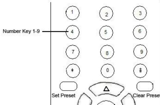
1、Preset setting : to set a preset position, the users should press the **【SET PRESET】** key first and then press the number key 0-9 to set a relative position, 10 preset positions in total are available.
